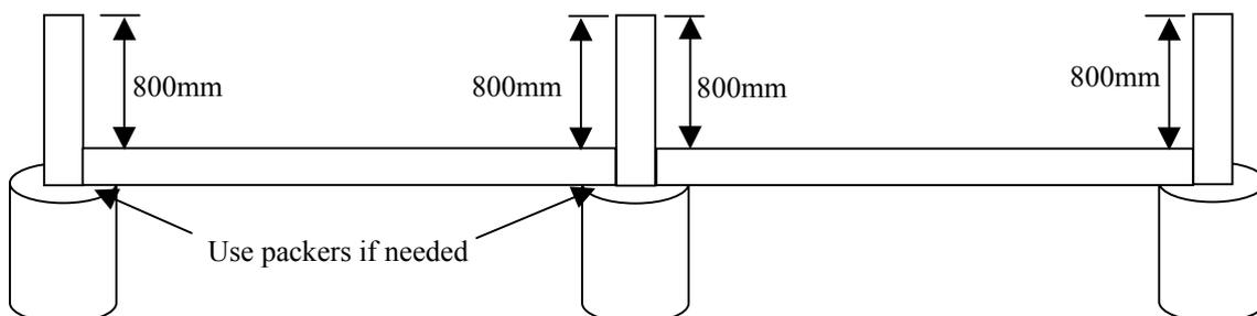
**Although you can slot your sleepers one day after the uprights were installed, it is not advisable to back-fill your wall for a few days as the concrete will not be fully cured.**
